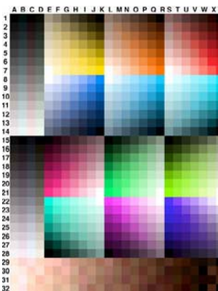
Figure 1. The WIR i-Star sRGBColorspace Target (v1.0) is a generic 800 patch test target for I* analysis. The target maps 12 hues with varying lightness and chroma, plus neutrals, near-neutrals, and skintone colors over the full tonal gradient and color gamut of the sRGB color space. Test targets can be made for other color spaces such as Adobe RGB and ProPhoto RGB (a large gamut colorspace also known as ROMM RGB).
