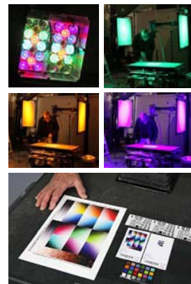
Fig. 2 Illumination from thirteen or more narrow wavelength LED's is used in a darkened room for sequential exposures with the MegaVision camera. Shown above is a standard 800-patch WIR i-Star image permanence test target printed on 8.5 x 11-inch photo paper together with two reduced-size “micropatch” WIR i-Star test targets.
