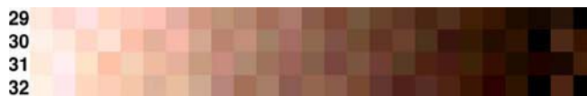
Figure 2. The human skintone colors section of the generic WIR i-Star target consists of 100 patches generated by adjusting the L* values of the measured LAB values for the “Light Skin” and “Dark Skin” color patches in the Macbeth ColorChecker chart. Photographs of people may range from very high L* values in specular highlight areas to very low L* values in deep shadow areas of the face. The number of skintone color patches and neutral/near-neutral patches relative to the total number of patches in the test chart provides a means of weighting these colors in the i-Star analysis. The skintone colors section of the target can also be analyzed separately as an i-Star “Region of Interest.”
